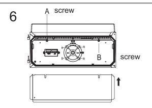
Put back the reflector and tighten the 2 screws
