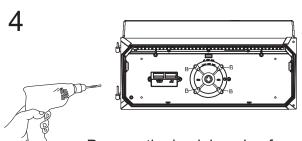
Prepare the back housing for mounting by drilling or knocking out the appropriate hole.
