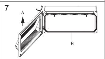
Put part A back onto the hinge of part B. Check the hinge for secure.
