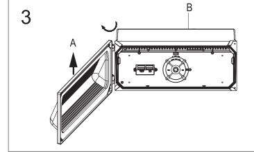
Separate part A and B and set part A aside.
