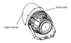
Put the light barrier on the lamp body
