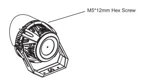
Use 6 pcs of M5\*12MM Hex Screw to lock the light barrier on the lamp body
