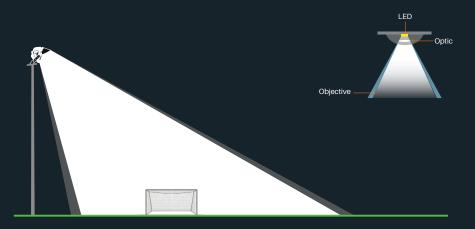
Engineered optics confine illumination to the play area, reducing spill light, glare and upward light.
