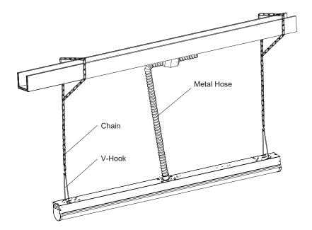
**LENS INSPECTION:** After installation check to make sure the lens is completely secure inside the lamp body and the end cap. Gently pull down on the lens to ensure it does not shift.
