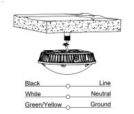
Screw the lamp and conduit pole together tightly
