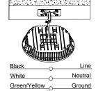
4. Slide lamp back into the connecting plate and fix the screw that is removed in step one
