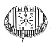
Fix the connecting plate onto the ceiling and put the wire through center hole
