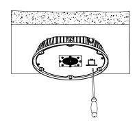
3. Put back the lens and check the function of sensor
