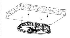
Remove 1/2" plug against the direction you intend to connect the conduit
